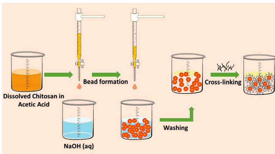
Figure 1. Schematic illustration of the preparation of cross-linked chitosan beads. [Color figure can be viewed in the online issue, which is available at wileyonlinelibrary.com .]
